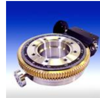
Fig. 2: The picture of M1 steering gear for horizontal motion. The center part is connected onto the GAMMA 10 installing port flange.
