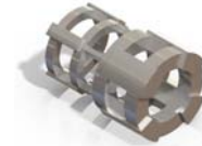
Fig. 2. An array of 3 quadrupolar coils.
