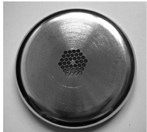
Fig. 2. Emission electrode with 36 openings.
